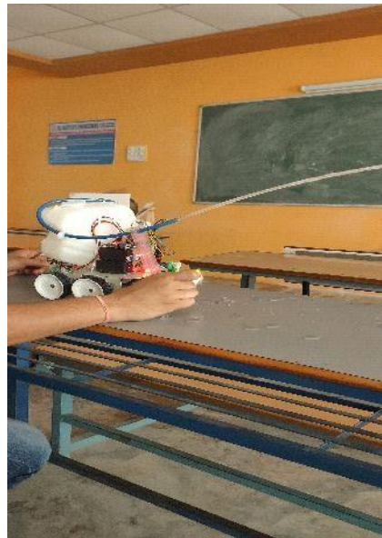
Fig.4: automaton sprinkling the water towards the fire
